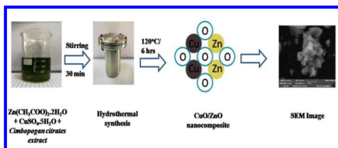
Scheme 2: Schematic illustration of preparation of CuO/ZnO nanocomposite by using hydrothermal method
